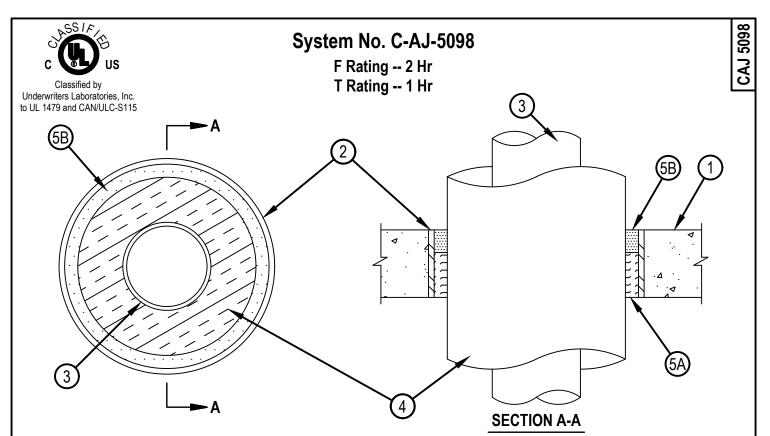
1. Floor or Wall Assembly — Min 114 mm (4-1/2 in.) thick reinforced lightweight or normal weight (1600-2400 kg/m3 or 100-150 pcf) concrete floor or min 6 in. thick reinforced lightweight or normal weight concrete wall. Wall may also be constructed of any UL Classified Concrete Blocks\*. Max diam of opening is 346 mm (13-5/8 in.).
